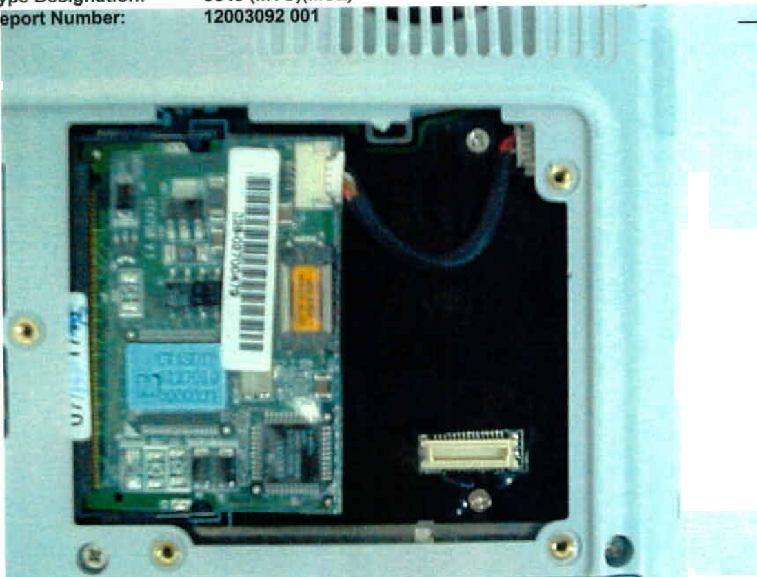
Mini PCI Modem Model "CTX 708" of "Creatix" installed (w/ insulator)
