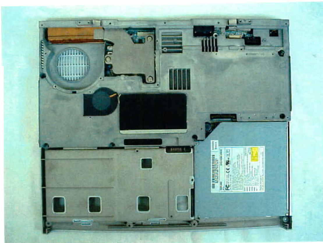
Internal Top View (w/ top enclosure, heatsink cover and LCD panel removed)
