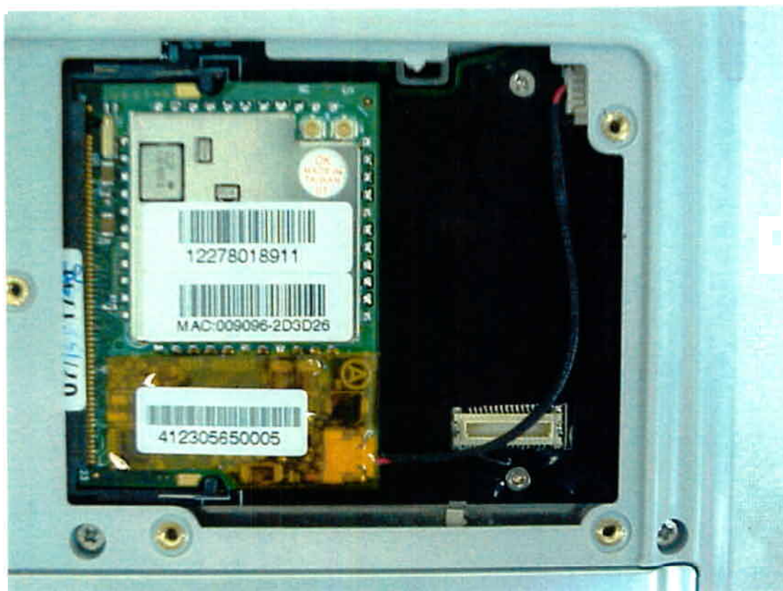
Mini PCI Modem "WLL030M" of "Askey" installed (w/ insulator)
