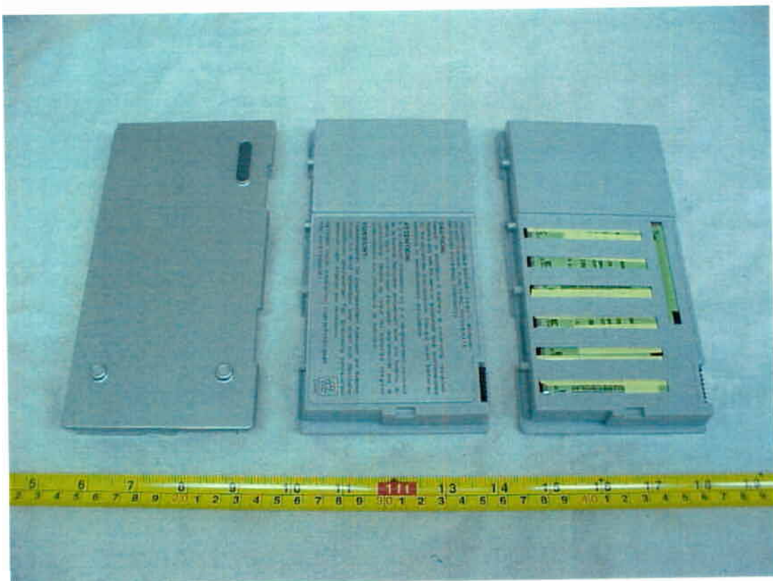
Battery Pack used for "8640" (top, bottom view, and w/ label removed)
